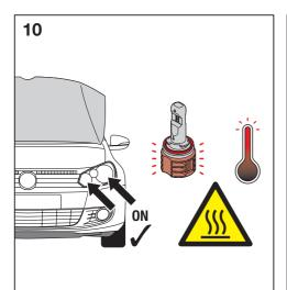
Do not stare at the operating light source.<sup>2)</sup> Caution! The cooling element on the back will heat when the headlamp is in operation.<sup>3)</sup>
