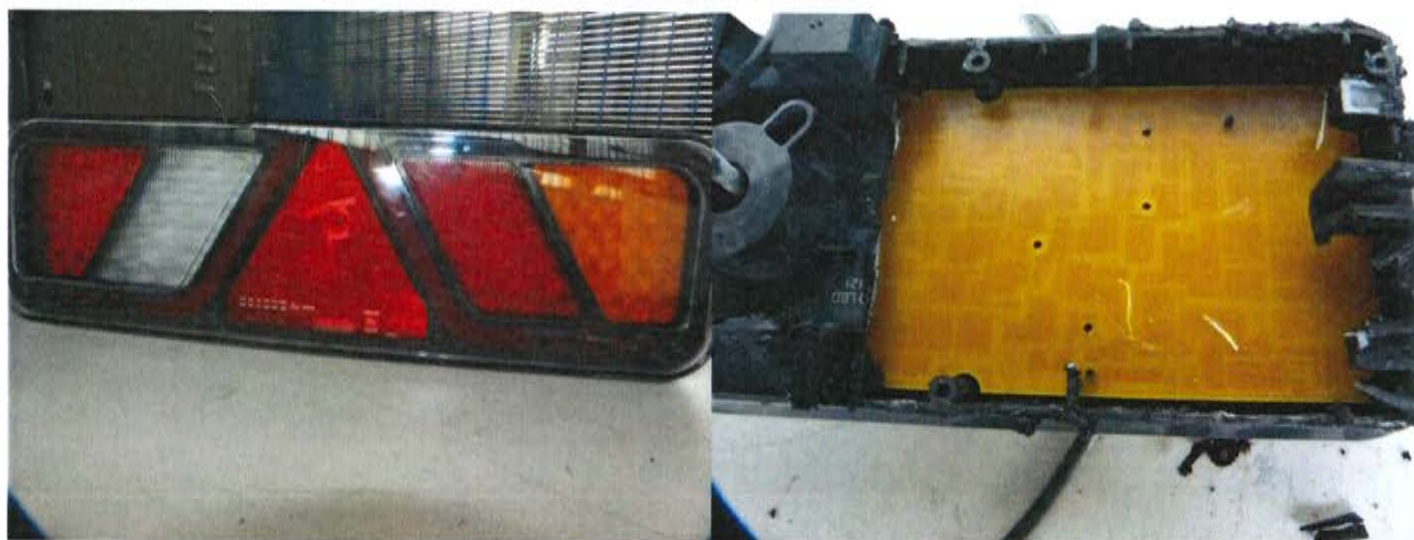
Photo. 8. Inspection of EUT 6649.01 after IP6X test
