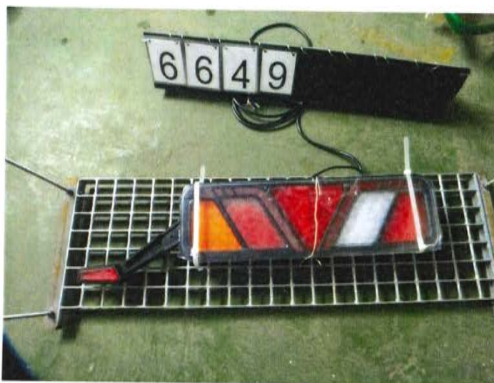
Photo. 2. EUT mounted on support before IPX8 test
