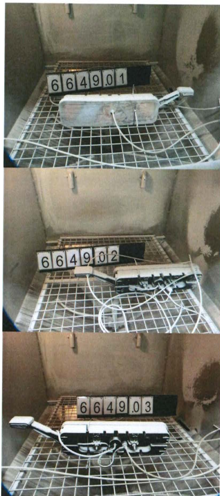
Photo. 7. EUT after IP6X test
