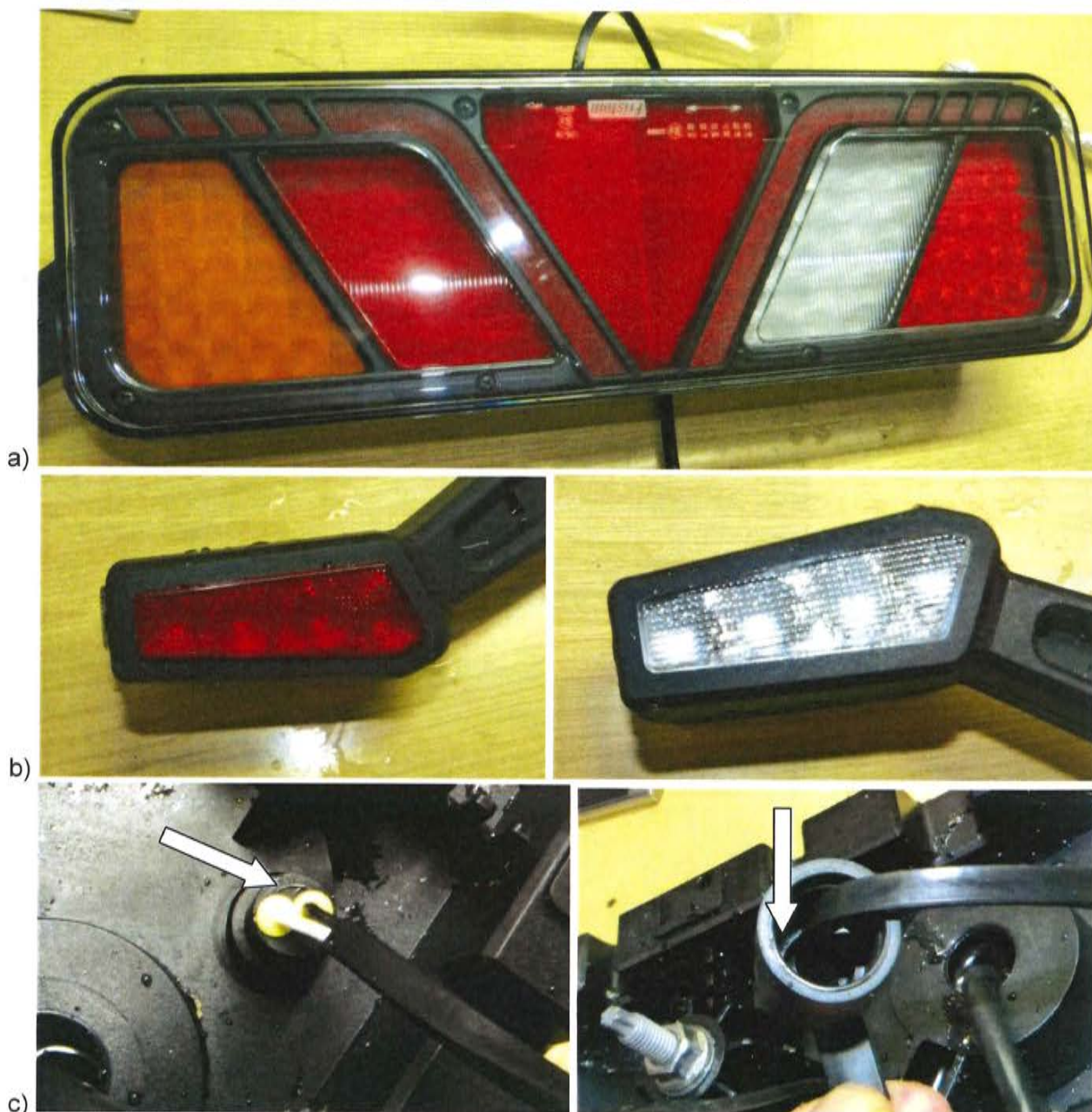
Photo. 4. Visual inspection after IPX8 test
