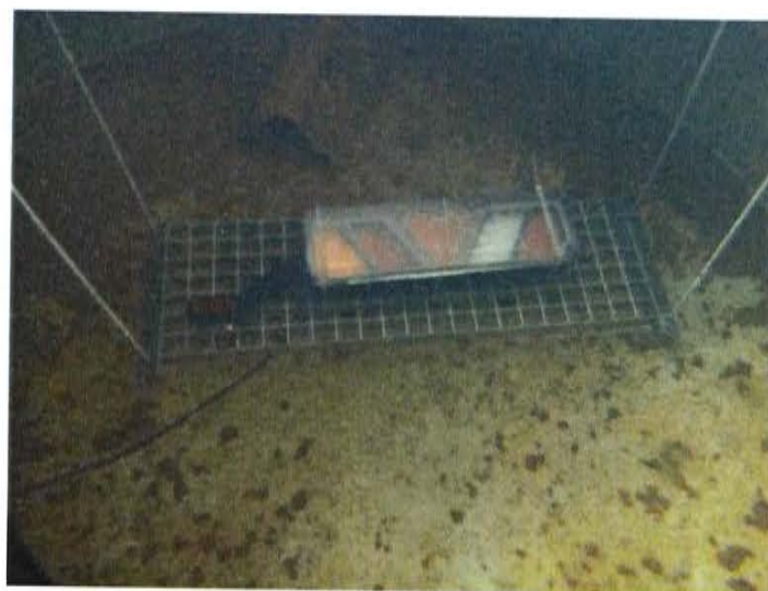
Photo. 3. EUT immersed in water
