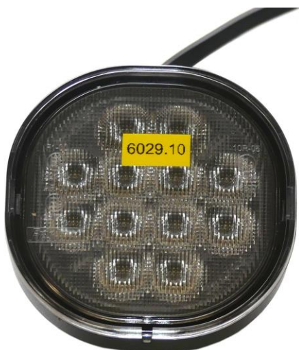
Photography 2: Sample 6029.10 – LED Lamp type FT-410 (to be tested on IPX8)
