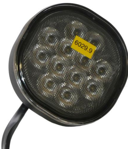
Photography 1: Sample 6029.9 – LED Lamp type FT-410 (to be tested on IP6X)
