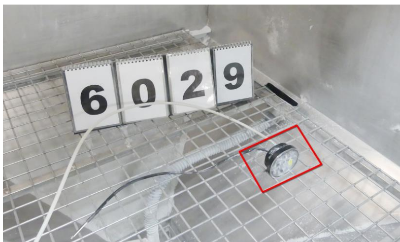
Photography 3: Sample 6029.9 – LED Lamp type FT-410 (marked with red line) during the IP6X test
