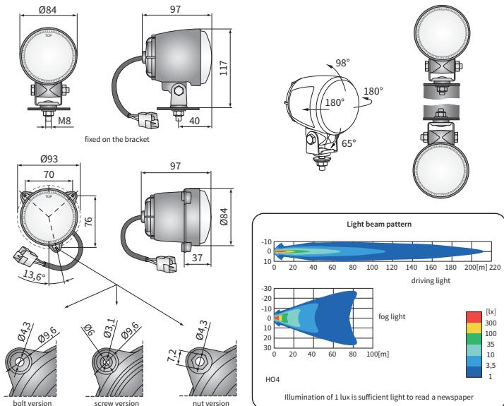
Mounting: factory prepared places, built-in to vehicle's recess, as a freestanding on the body work. Versions with the bracket can be installed on a vehicle in an upright or upside-down position. It is possible to install needed connectors on wire (on request).
