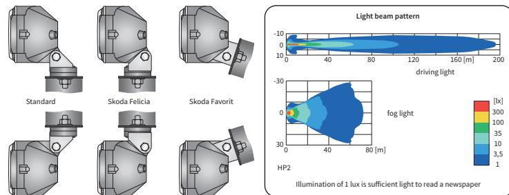
To be mounted at the front of the car or truck. They can be installed in an upright or upside down position.
