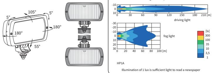
To be mounted at the front of the car or truck. They can be installed in an upright or upside down position.
